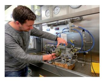
Sebastian Barheier, Lufthansa Technik Project Manager Components Lockheed L-1649A, takes a close look at the test installation, developed in cooperation between Lufthansa Technik and RTG. (Wolfgang Borgmann)
